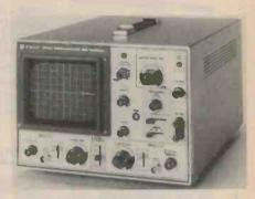
PARAMETERS PTY LTD, 68 Alexander St, Crows Nest, NSW 2065. (02) 439 3288. They handle Trio oscilloscopes which are among the most popular general-purpose and service types. Currently the most popular in the range is the CS-1560AII, a 15 MHz dual-trace model with easy TV sync triggering facilities. It has a sensitivity range of 10 mV/div to 20 V/div.
