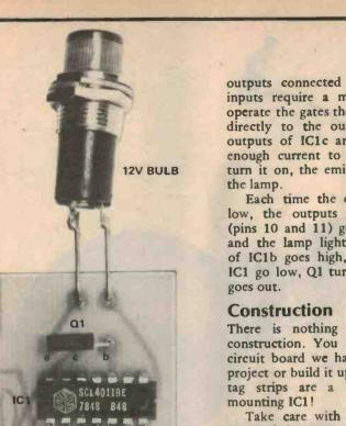
To turn a lamp on and off requires a little more circuitry. We couldn't connect the lamp at the output of IC1b as it would rapidly discharge C1 at the wrong time! To switch the 150-200 mA required by the lamp, we use a transistor to amplify a small current supplied to its base, the lamp being connected between the emitter and the negative side of the supply. This sort of circuit is called an "emitter
