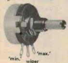
The common potentiometer — a variable resistor. Terminal markings are standard for a volume control.
